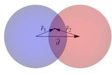
Recall that the electric field of a uniformly charged solid sphere with charge density  $\rho$  is given by  $\vec{E} = \frac{\rho r}{3\epsilon_0} \hat{r}$  (as can
