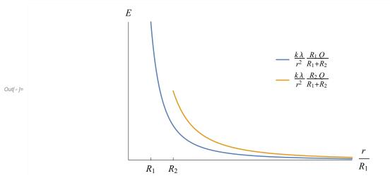
So only a very tiny bit of charge goes onto the wire, and all the remaining charge will stay on the two spheres. The only remaining point is to discuss our initial assumptions: that only a tiny bit of charge goes onto the wire and that this charge is uniformly distributed along the wire. The first point is discussed in Problem 3.10 where it is shown that a thin wire has essentially zero capacitance. The second point is discussed in Problem 3.5, which is definitely
