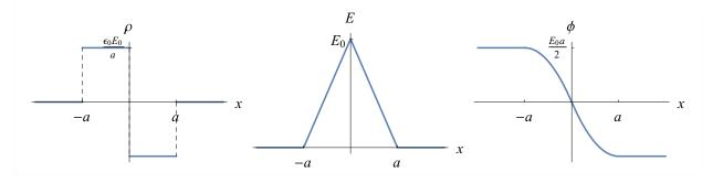
As a double check, at x = 0 the two infinite slabs act effectively like sheets with charge densities  $\pm \sigma = \pm \rho a$ . They create a field pointing to the right with magnitude  $\frac{\sigma}{2\epsilon_0}$ , so the total field is  $2 \frac{\rho a}{2\epsilon_0} = \frac{\rho a}{\epsilon_0}$ . Since we found that
